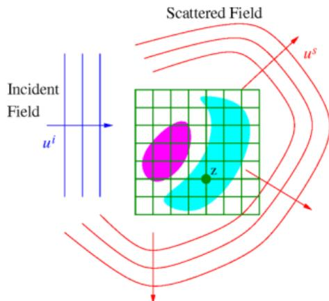
Figure: Shape Reconstruction via Sampling in a Grid
