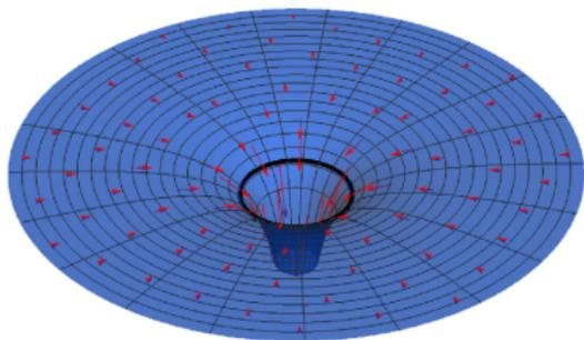
Figure: View of an Acoustic Black Hole: Technique for Passive Vibration Control
