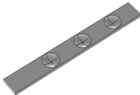
Figure: A schematic of a plate with three equally spaced neutralisers for vibration damping
